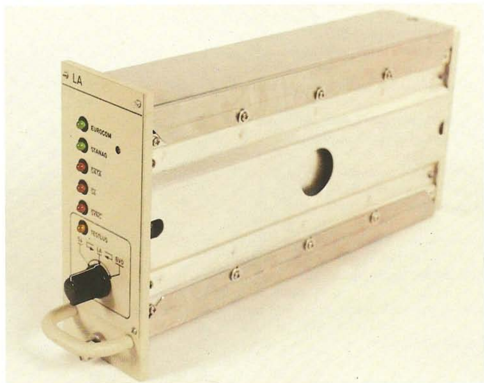
Fig. 13. Line terminating unit
