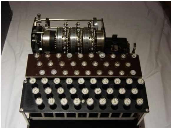
Photo 1: A133 without cover. Source: FRA
