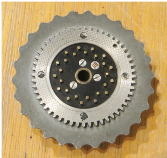
Figure 5 and 6. Side views of rotor III from Enigma G 350 in the collection of Försvarets Radioanstalt. Photo © 2019 Anders Wik, courtesy of FRA.
