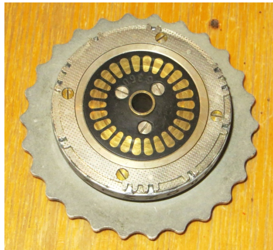
Figure 5 and 6. Side views of rotor III from Enigma G 350 in the collection of Försvarets Radioanstalt. Photo © 2019 Anders Wik, courtesy of FRA.
