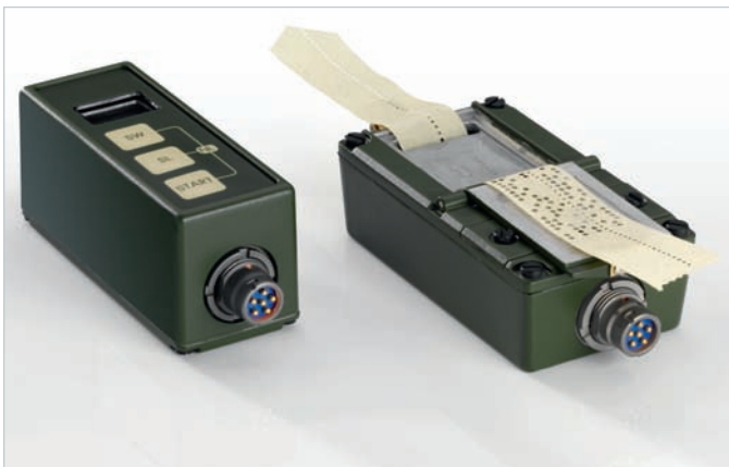
Fill devices for manually loading encryption keys.
